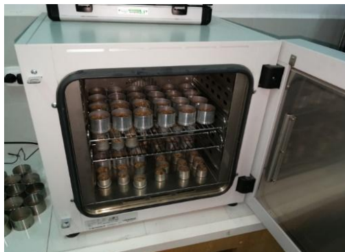
Fig. 4 Samples subjected to drying in the oven FD 53 model with forced ventilation
